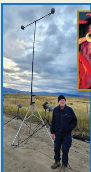
CAS Associate Dan Dugan having trouble in the field: "Nature recording fail in Sierra Valley, CA. Wind is bending the boom. After the tripods blew over, I had to spread the legs wide to keep them up. The birds were still singing but I couldn't get a listenable recording. But if you don't try, you'll surely get nothing!"
